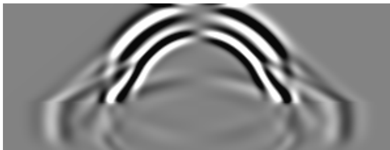
Fig. D.10 Snapshot after 0.4 seconds, note the two head waves.
