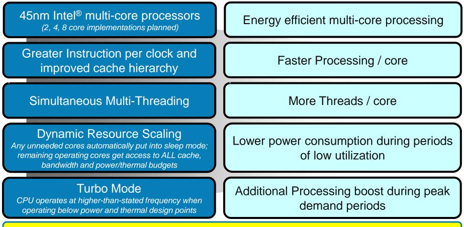
FASTER cores ... MORE cores/threads ... DYNAMICALLY ADAPTABLE
