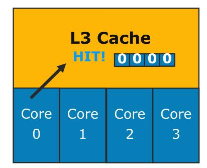
Core valid bits limit unnecessary snoops
