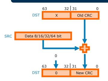
One register maintains the running CRC value as a software loop iterates over data. Fixed CRC polynomial = 11EDC6F41h
