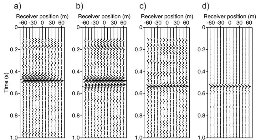
**Figure 2** Retrieved virtual reflection response from a) the base and b) the repeat experiment using a different noise-source realization. c) The extracted time-lapse signal. d) The extracted time-lapse signal when the noise-source realization in the base and repeat experiments is the same.
