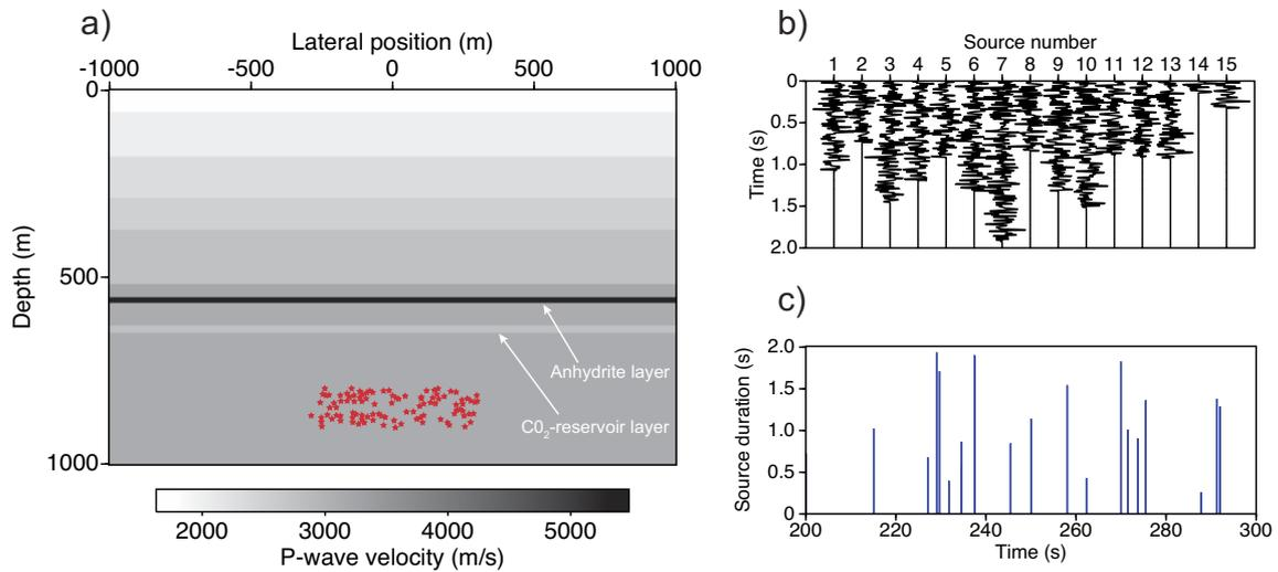
**Figure 1** Modelling of the passive body-wave noise measurements. a) Velocity model with red stars indicating a random distribution of 100 sources in the region between  $x=-300$  m and  $x=300$  m and between  $z=800$  m and  $z=900$  m. b) The signatures of 15 out of the 100 sources. c) The triggering sequence of the modelling between  $t=200$  s and  $t=300$  s.
