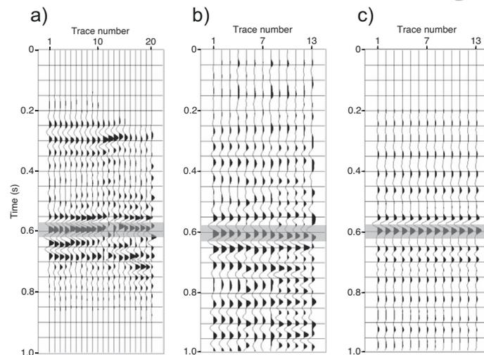
**Figure 4** a) Ketzin field-data stack profile using active sources and a receiver line at the surface. b) Auto-correlation result using one day of noise recorded on the vertical component of the buried geophones. c) Auto-correlation panel from modelled passive data. The three panels are filtered to the same bandwidth. The gray stripes indicate the candidate location of the K2 reflector.
