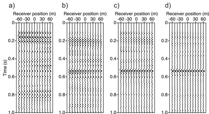
**Figure 3** The time-lapse reflection signals after application of ANSI for a) 20 noise sources, b) 40 noise sources, c) 80 noise sources and d) 160 noise sources. The sources are confined to the region between  $x=-150$  m and  $x=150$  m and between  $z=800$  m and  $z=900$  m in the model.
