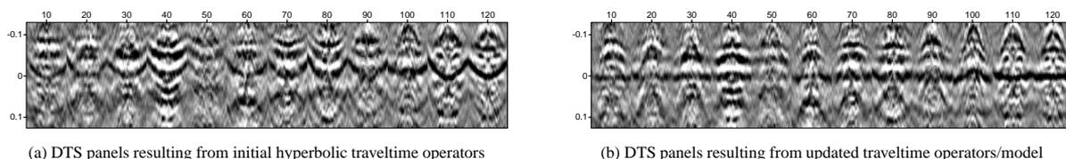
**Fig. 1:** Example of 2D Differential Time Shift (DTS) panels along a boundary in the North Sea data set, that shows the misfit between the modeled operator in the updated model and the Common Focal Point (CFP) gather over the offset along the seismic line. If the modeled operator and the CFP gather coincide, the event of interest is aligned at  $t=0$ .
