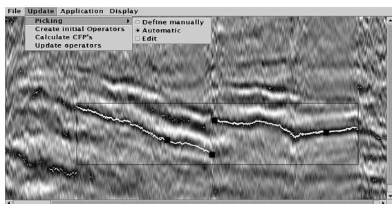
**Fig. 2:** Zoom of the stacked section from the North Sea data with the boundary indicated by a track overlay (white), and the user determined picks denoted by the black squares.
