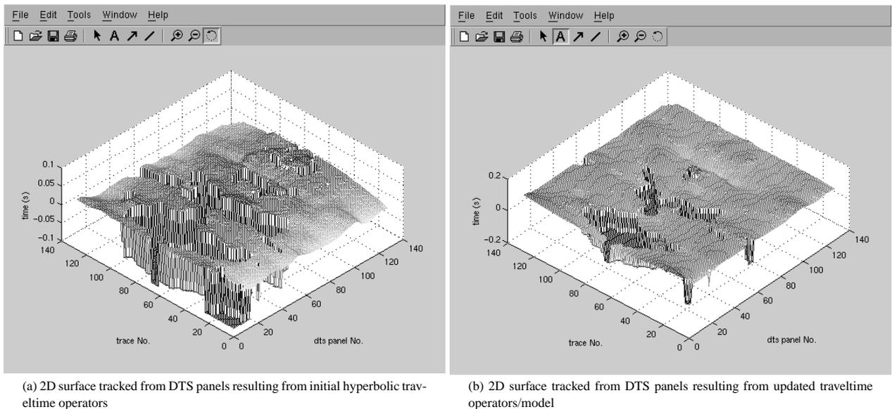
**Fig. 4:** The 2D surface that was automatically tracked from the 3D data volume built up from all the 2D DTS panels along the same boundary.
