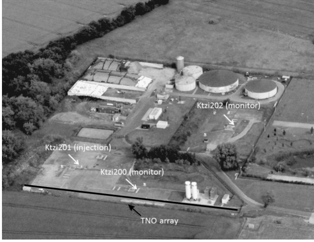
Figure 3. View of the injection site (courtesy of GFZ). The black solid line denotes the approximate 120-m-long east–west-oriented line formed by TNO’s surface sensors. The locations of injection well Ktzi201 and the two monitor wells Ktzi200 and Ktzi202 are indicated by the white arrows.
