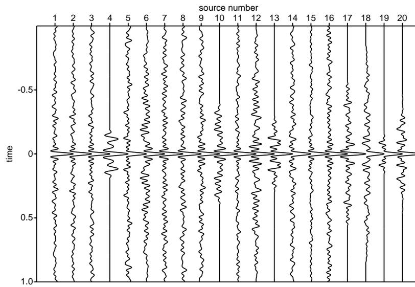
Figure 11: *Auto-correlated random source signatures with varying source duration normalized to the maximum amplitude per trace. The longest signals (source numbers 11 and 15) have the highest auto-correlation peak and best S/N ratio. The script `Figure17_19AppendixA.scr` in the `FiguresPaper` directory reproduces the pictures.*
