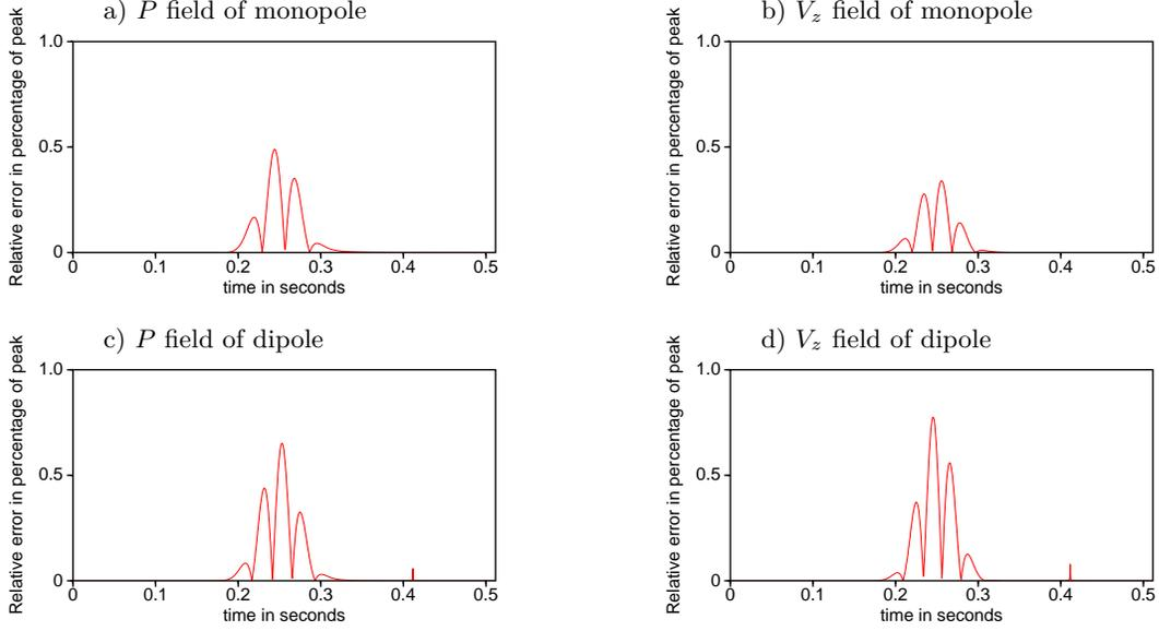
Figure 24: Difference between the analytical Green's function and the finite-difference result in an acoustic medium for monopole and dipole sources for  $P$  and  $V_z$  recorded fields. The difference is shown as percentage of the maximum peak in the analytical Green's function. A grid spacing of  $\Delta = 2.5$  m is used. The script `FigureGreenDxAppendixA.scr` in the `FiguresPaper` directory calculates the data and reproduces the pictures.
