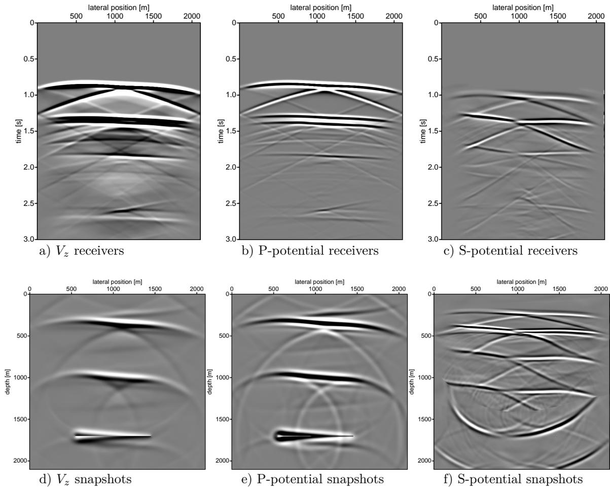
Figure 18: Panel a, b, and c show three different types of receiver measurements at depth  $z = 400$  m. Panel d, e, and f show three snapshots at  $t = 0.5, 0.9, 1.3$  for different types of wavefield components.
