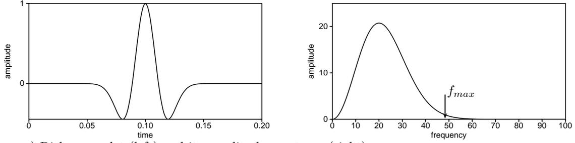
a) Ricker wavelet (left) and its amplitude spectrum (right).
