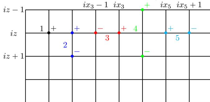
Figure 13: Implementation of different source orientations on the grid. The different numbers (colors) show the options of parameter `src_orient=`. The + and - symbol represent the sign of the source amplitude added to the computational grid.
