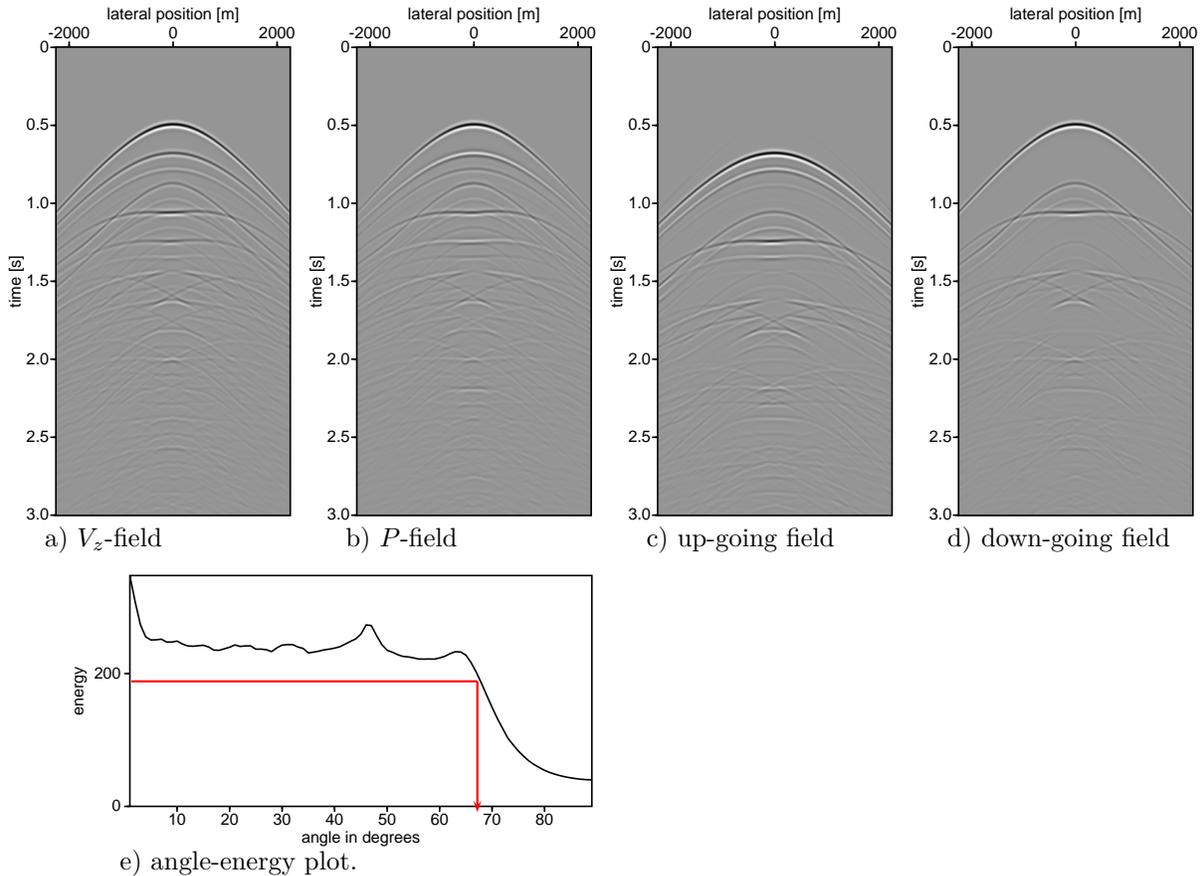
Figure 15: The  $P$  (a) and  $V_z$  (b) fields and the decomposed up (c) and downgoing (d) fields from example `demo/decomposition.scr`. Selection of maximum angle (e) to filter the decomposition operator in  $k_x - \omega$  domain.
