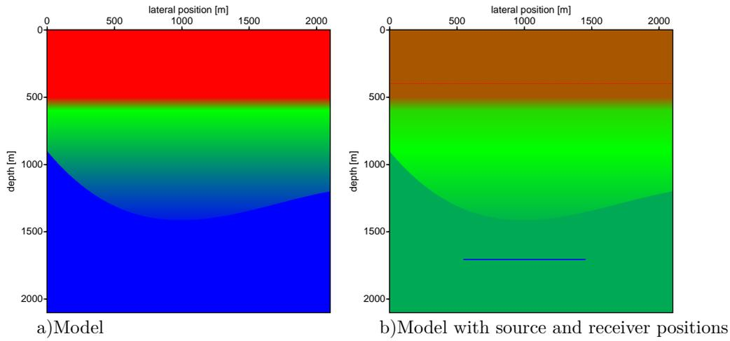
Figure 17: Gridded model used to model a plane wave at  $x = 1000, z = 1700$ . The receivers are placed at depth level  $z = 400$  m, just outside the taper area at the top, which ends at  $z = 360$  m. Source (blue dots) and receiver (red dots) positions are shown in b).
