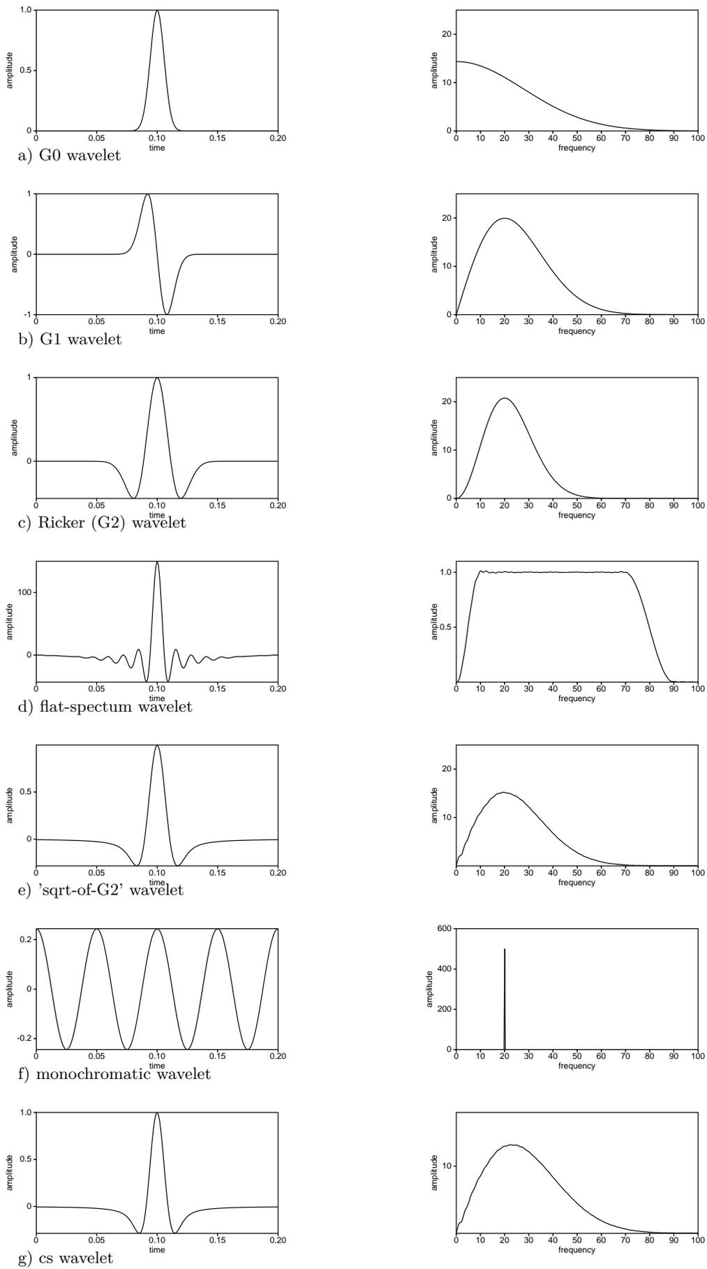
Figure 30: Time and amplitude spectrum of the wavelet types generated by the program `makewave`.
