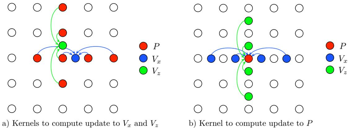
Figure 2: The compute kernels showing the grid points needed to update the  $V_x$  and  $V_z$  (a) and  $P$  (b) wavefields. The wavefields all have a unique grid position. A staggered grid implementation has been used. This means that the grids of the  $V_x$  and  $V_z$  wavefields are positioned in between the  $P$  grid.
