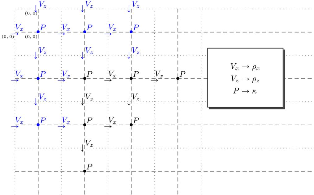
Figure 4: Acoustic staggered calculation grid for a fourth-order scheme in space.  $V_z, V_x$  represent the particle velocity of the wavefield in the  $z$  and  $x$  direction, respectively, and  $P$  represent the acoustic pressure. The blue fields are auxiliary points used to calculate the black field values. Those blue points are not updated and initialized to zero. On all sides of the model a virtual  $V_x$  or  $V_z$  layer has been added for proper handling of the edges of the model.
