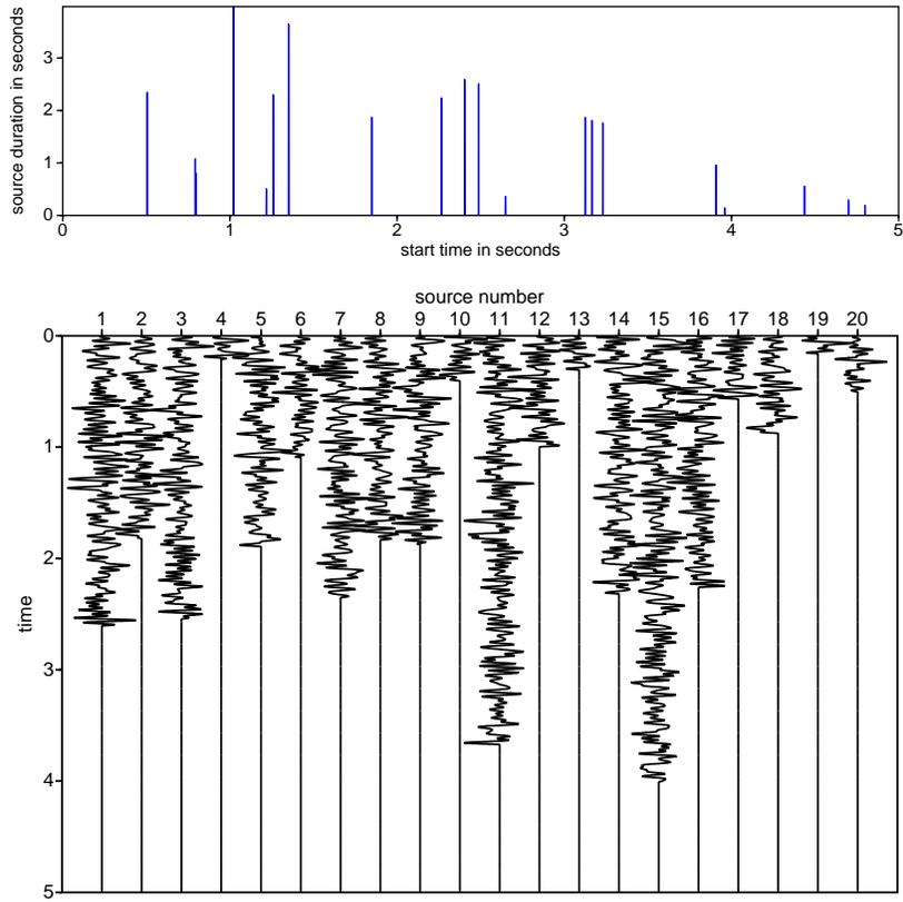
Figure 9: *Random source signatures with varying source duration (top picture). Note that the sources start at random times in the interval  $t_{src1} = : t_{src2} =$ . The script `fdelmodc_rand.scr` in the demo directory calculates the data and `eps_for_manual.scr` reproduces the pictures.*
