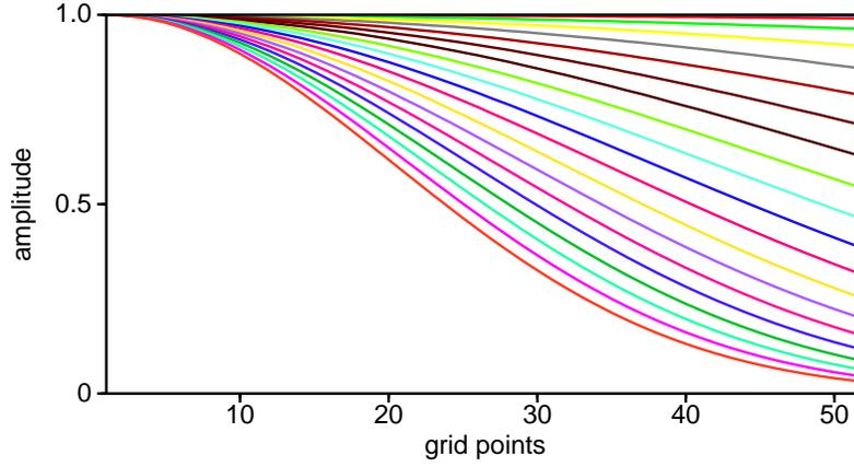
Figure 7: The boundary taper as function of the `tapfact`= parameter is shown. The red line with the highest amplitude has `tapfact=0.1`, each line with a lower amplitude has a tap fact 0.1 larger (e.g. the green line has 0.2, the yellow line 0.3).
