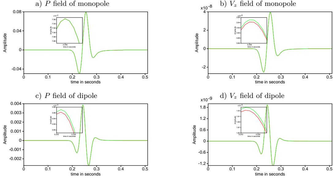
Figure 23: Comparison of Green's functions in an acoustic homogeneous medium for monopole (top) and dipole sources (bottom) with pressure ( $P$ ) and particle velocity ( $V_z$ ), left and right, respectively, recorded wavefields. The onsets show the differences for the positive peak of the wavelet, the lower line represents the finite-difference result. The script `FigureGreenAppendixA.scr` in the `FiguresPaper` directory calculates the data and reproduces the pictures.
