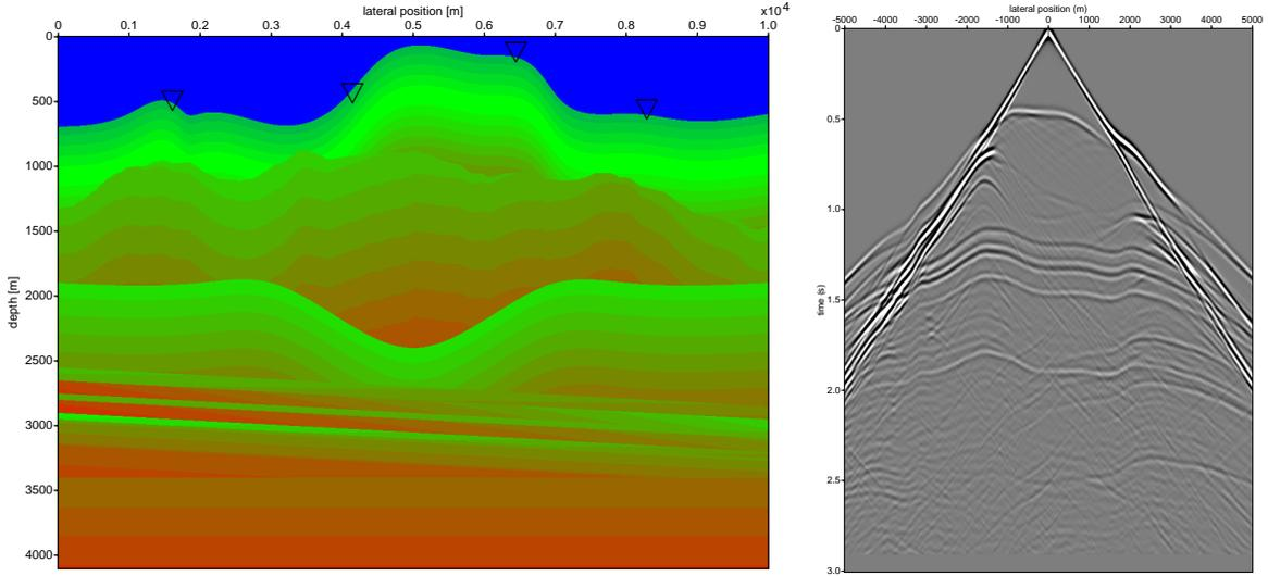
Figure 22: The receivers are placed from -5000 m to 5000 m at every 20 m on the topography. The modeled reflection response, for a source at 5000 m placed on the topography, is shown in the right picture.
