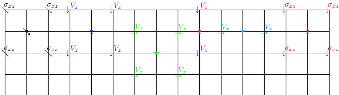
Figure 16: Receiver interpolation options in the elastic staggered calculation grid.  $V_z, V_x$  represent the particle velocity of the wavefield in the  $z$  and  $x$  direction respectively and  $\sigma_p(\sigma_{xx}$  or  $\sigma_{zz}), \sigma_{xz}$  represent the stress fields.
